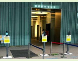
Those standing temperature measurement cameras installed at the front of the elevator hall can accurately measure in as little as 0.2 seconds even with a mask on by using the AI face detection technology.
